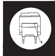
Stand-Off Lugs Minimize Solder-Creepage
